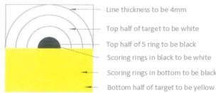
Line thickness to be 4mm Top half of target to be white Top half of 5 ring to be black Scoring rings in black to be white Scoring rings in bottom to be black
